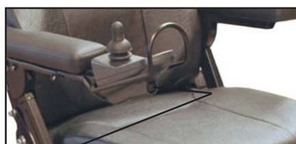
Connect the charging plug to the 3-pin socket on the joystick.
